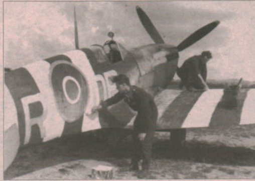
Leading Aircraftman Ken Allenby (next to fuselage) and Leading Aircraftman Stan Rivers (on starboard wing), both 'erks' with No. 411 'Grizzly' (F) Squadron apply generous amounts of paint to a Supermarine Spitfire L.F. Mk. IXb the day prior to the Normandy invasion. All allied aircraft operating over Normandy were given the cosmetic treatment to ensure there would be no problems mistaking them for enemy aircraft. The photo was taken at their home base, R.A.F. Station Tangmere, Sussex.
