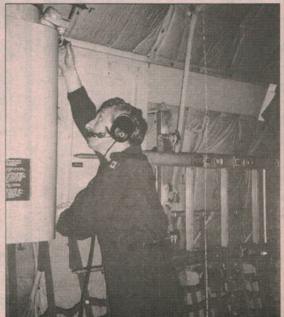
Loadmaster MCpl Chris Young checks the hydraulic quantity during an Op Alliance flight.
