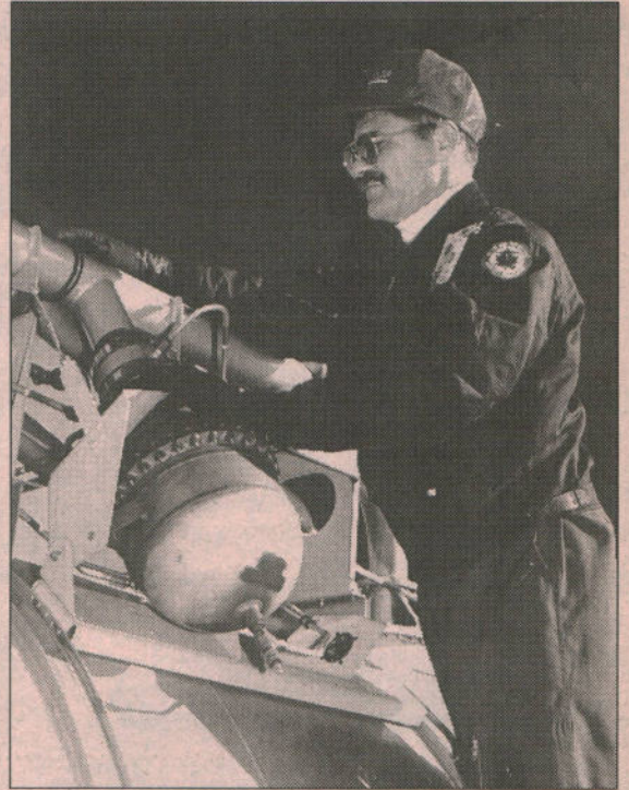
Sgt Mackey does a visual check on the 3600 gallon Fuselage Tank.
