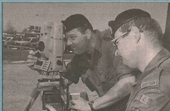
Sgt Al Podzorski and Sgt Wim Bokhout of 1 Construction Engineering Unit use a "Total Station" to check elevations while taking a topographical survey along East Road near Wing Headquarters on 18 May 1995. The survey work is being done in preparation for the repaving of roads in front of Wing Transport and Wing HQ. The repaving will be contracted out by Wing CE, and should take place later this summer. (Photo by Cpl Stephane Gervais, 17 Wing)
