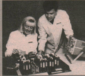
Spar technicians Jocelyne Vadeboncoeur and Benoit Bédard assemble the receiver or transponder for Sarsat. The transponder receives and retransmits distress signals.
