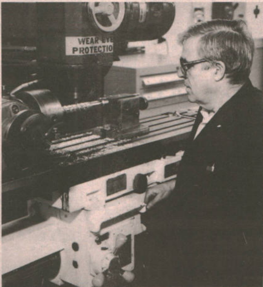
Mr. Gerry Saumure, machinist, is milling a spiral flute on a candlestick. He is wearing safety lens prescription glasses.
