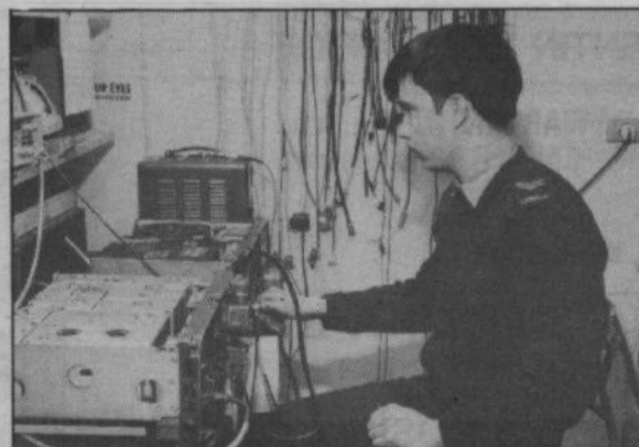
Corporal C.J. Young, a 221 Radio Technician from 733 Communications Squadron, gains practical experience performing checks on a GRC-106 radio set in the BML Communications Repair Shop.
