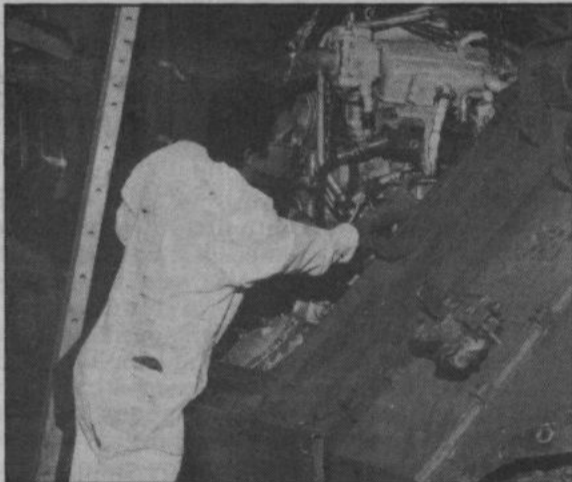
Yogi Barmeda, a VHE 9 mechanic, removes the engine assembly from an M-113 Armoured Personnel Carrier.
