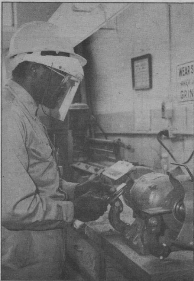
Mel Flake sharpens a chisel on a bench grinder, using guard and full-face shield.
