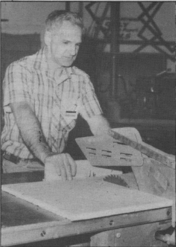
Carpentry — Dusty Miller checks safety guard on circular bench-saw.
