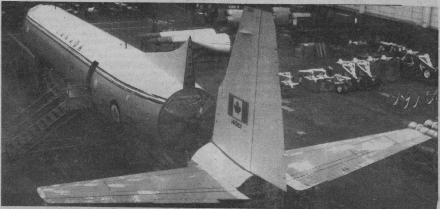
The completed tail section bearing the number "140101" is aligned with the fuselage at the beginning of the final assembly line.
