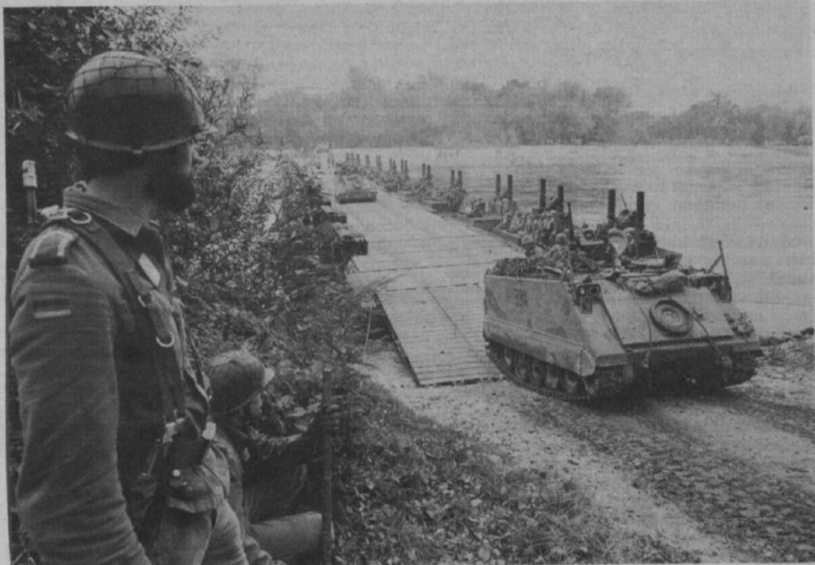
Armoured personnel carriers of 3 Royal Canadian Regiment (3 RCR) roll across the Danube river on a floating bridge constructed by II German Corps engineers during Exercise Blau Donau. The exercise is one of several in the Autumn Forge series scheduled by the Supreme Allied Commander Europe.
