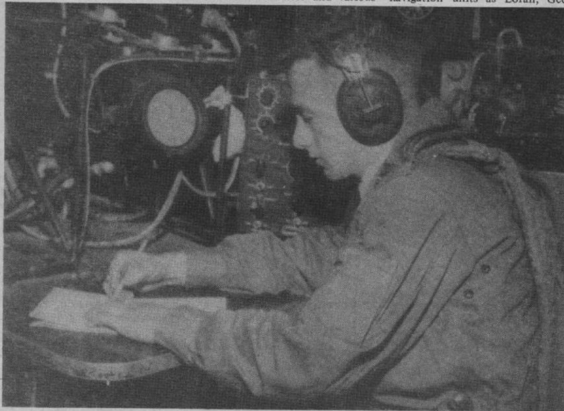
F/C G.L. McPhee, student at the Long Range School, uses the APS 33 Airborne Radar on a training flight.
