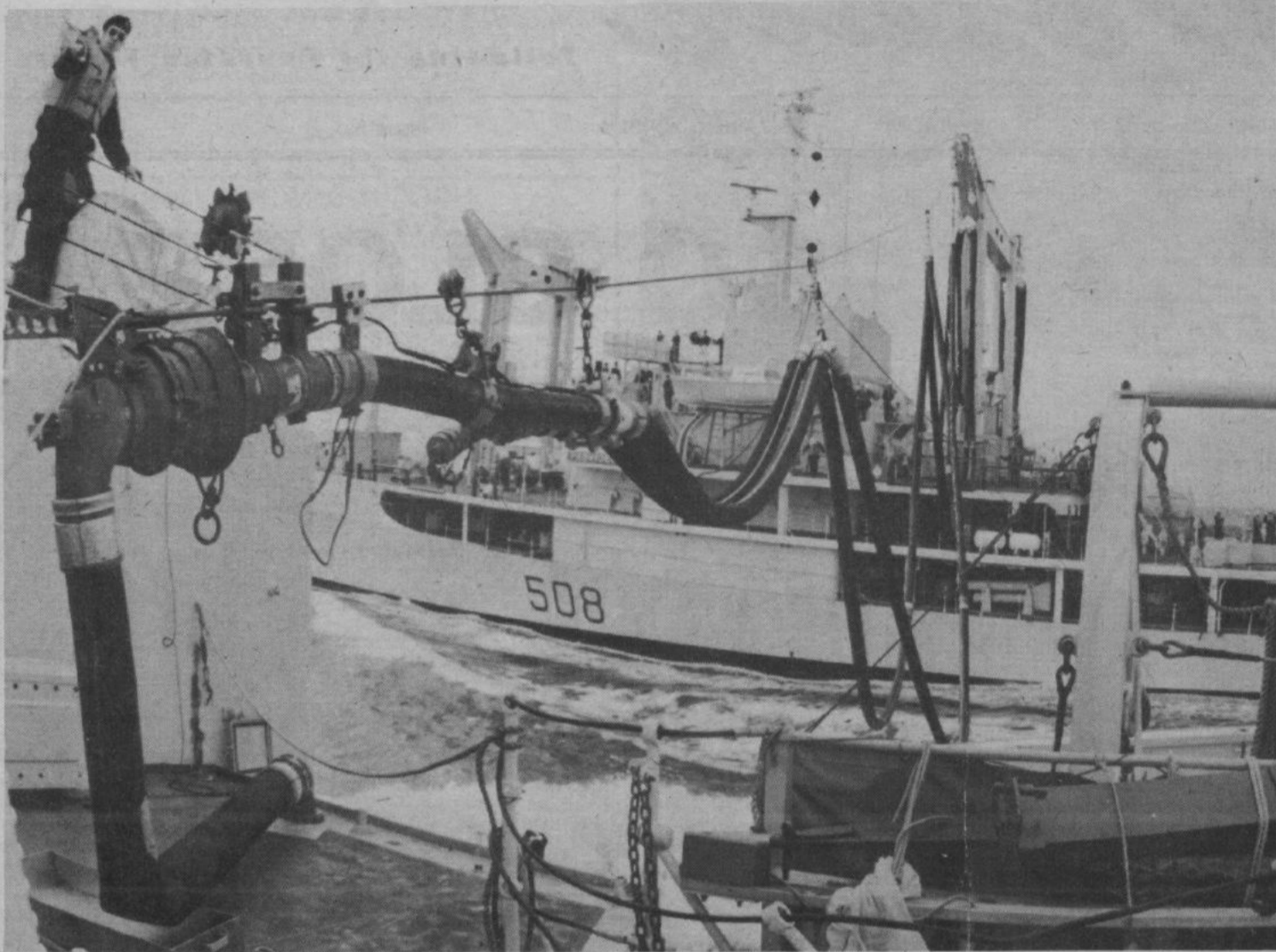
HMCS Restigouche of the Esquimalt-based 2nd Canadian Destroyer Squadron receives a refueling in mid-Pacific from Maritime Forces Pacific support ship HMCS Provider. The fuel oil is carried in a hose suspended from a span wire from the top of Provider's "goal post" and served inboard in the destroyer. The two warships and a second squadron destroyer (background) HMCS Kootenay are currently on a lengthy operational deployment in the Southwest Pacific. They return home May 5th. (CANADIAN FORCES PHOTO)
