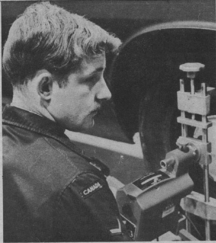
Toronto - Private David Lindbeck of 2 PPCLI carries out vehicle front end alignment during Vehicle Technician course at Canadian Forces School of Aerospace and Ordnance Engineering, Borden. Canadian Forces vehicle technicians are responsible for the maintenance, servicing repair and overhauling of forces land vehicles. (CANADIAN FORCES PHOTO)
