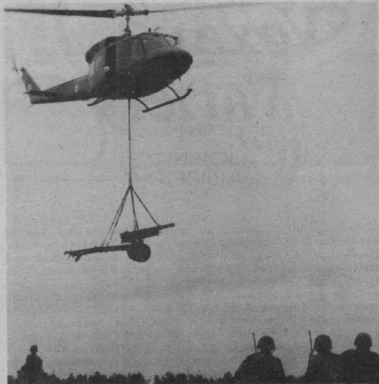
A Canadian Forces Huey helicopter lowers a 155-mm gun howitzer into position while the gun crew waits for the drop. The action took place during Exercise Mobile Warrior at Canadian Forces Base Petawawa. (CANADIAN FORCES PHOTO)
