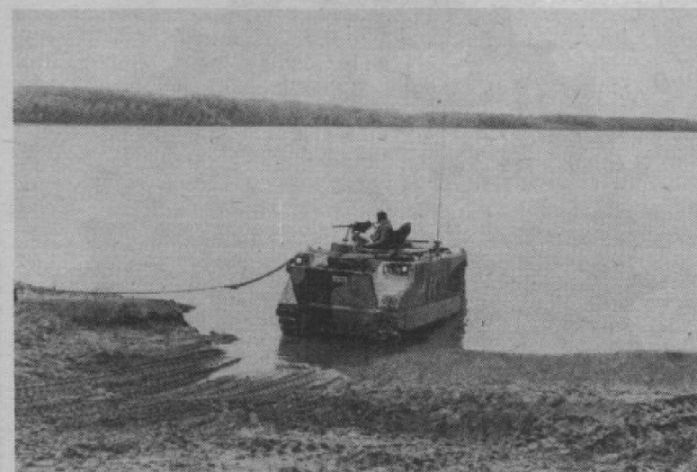
Prior to the swimming of the APC, a float test is done. The tow cable is attached to a recovery vehicle to counteract the submarine effect.
