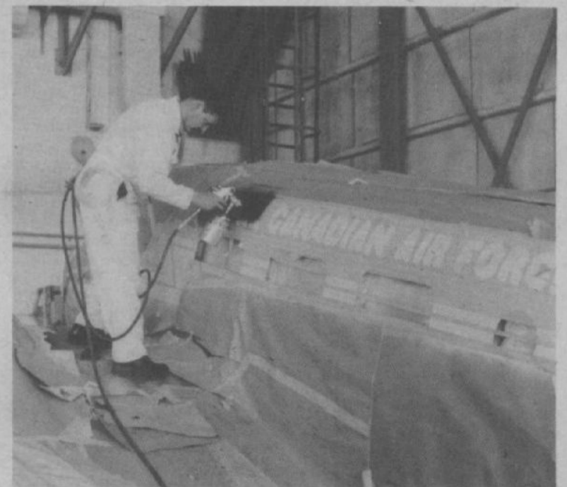
Corporal Chester MacDonald of the Base Aircraft Refinishing Section applies the base coat of black enamel to the Royal Canadian Air Force markings on the Expediter aircraft, starting one more of the many steps necessary to restore the airframe to display condition.
