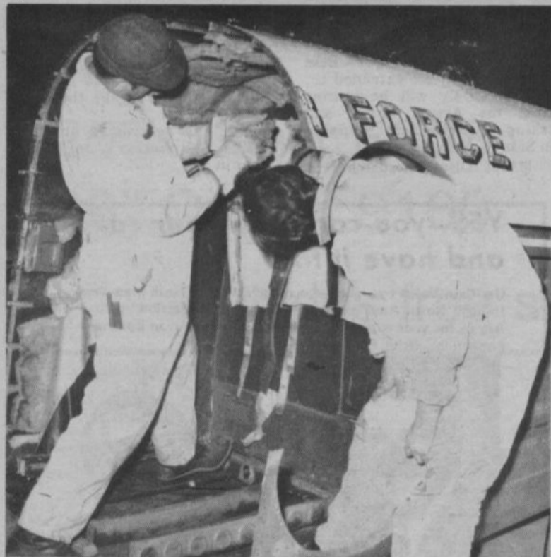
12 March Cpl Carlson uses an air drill to remove rivots to separate the aft section from the centre section
