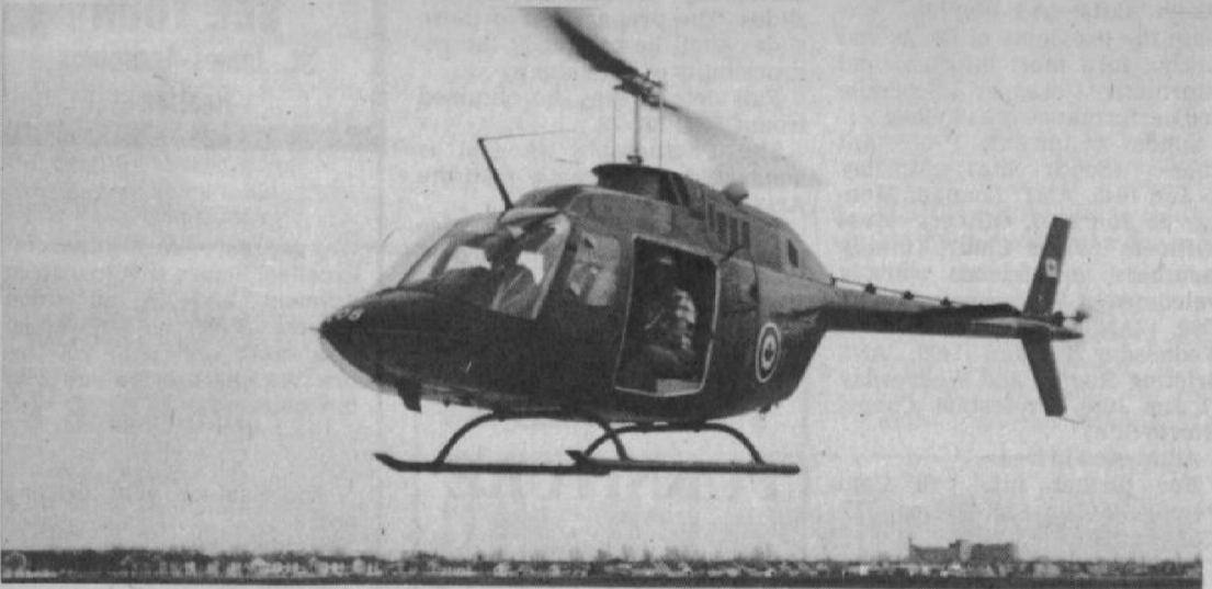
CH-136 KIOWA A four-seat light observation helicopter built by Bell Helicopters, is used primarily for advanced pilot training at CFB Portage, Manitoba. It can also be used for armed reconnaissance and medical evacuation, as well as in an observation role. Although they are based at C.F.B. Portage, Winnipeg residents will be very familiar
