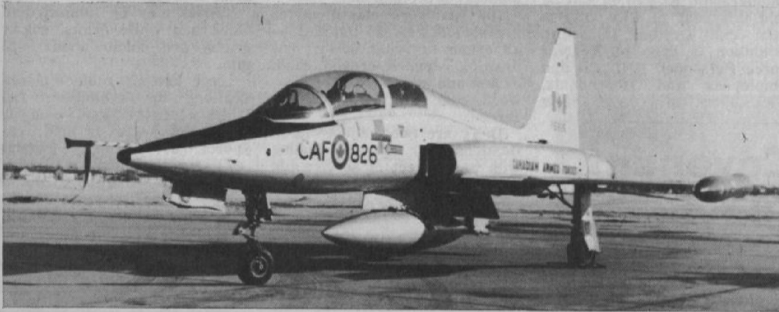
THE CF-5 FREEDOM FIGHTER is a twin-engine supersonic jet tactical fighter, designed for missions in close support of troops, interception of enemy aircraft,
