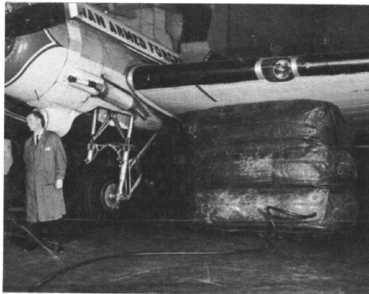
NOT A WATER BED, but this aircraft lifting device could easily lift one using air pressure. Sgt. Ron Swayze gives the briefing on the use of the air bag.
