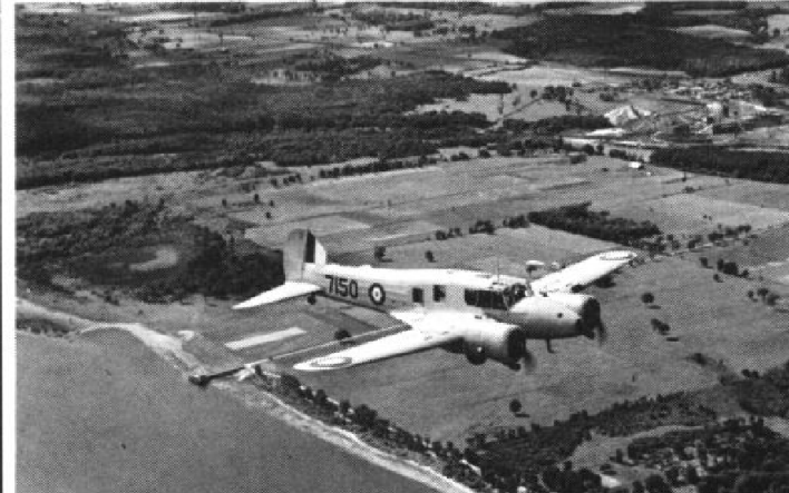
ANSON — Named after a famous British admiral of yore, the Avro Anson had its debut in RAF coastal command at outbreak of the second world war. Flapping, wiggling and jiggling it seemed in every part, the Anson nevertheless could take amazing amounts of punishment, could easily turn inside enemy fighters with its low top speed of 188 mph. In Canada from 1940 onwards, different models of the Anson were used in the British Commonwealth Air Training Plan to train more than 20,000 aircrew. The Mark V (175 mph) was used by the RCN as a light transport and training aircraft 1945-47 and only within the past couple of years did the RAF lay up the Anson.
