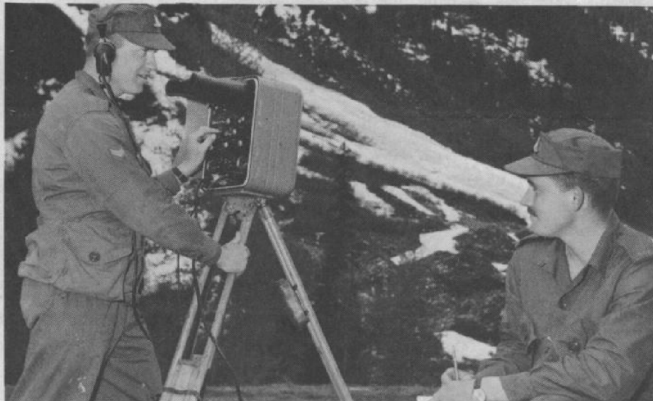
WINNIPEG, MAN., JAN. 31, 1968 — Bombardier Ralph Jervah and Bdr Ken Hamilton survey a distance with a Micro-Distancer in the rugged Rogers Pass. Both members of the Survey Troop, in co-operation with the Departments of Natural Resources and Northern Affairs, were part of an exercise to survey avalanche Control gun positions.
