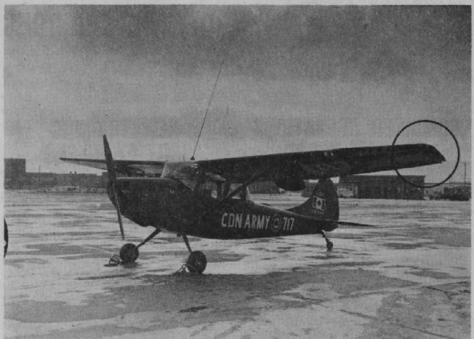
Things were quiet around 16 Hangar at noon last Wednesday, when there arrived an Army L19E-717. The aircraft, flown by Capt. MacGregor and Cpl Mason of Shilo, had struck a wire stretched between two hills near Falcon Lake. The propeller, engine nacelle and port wing were damaged, but Capt. MacGrgor was able to control the aircraft and flew 90 miles to a safe landing at Winnipeg. The plane was on an authorized low level spotting exercise, and the personnel of Stn Winnipeg congratulate the crew of 717 for the skill displayed in saving the crippled plane.
