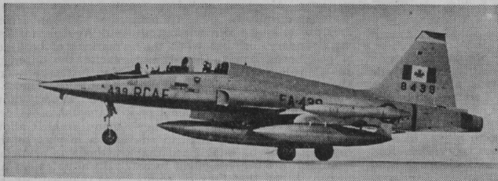
VERSATILE — The CF-5 is considered one of the most versatile aircraft in existence. It can be used for the close support of ground troops, aerial reconnaissance, air-to-air combat, supersonic interception, or as either a tactical fighter or trainer.
