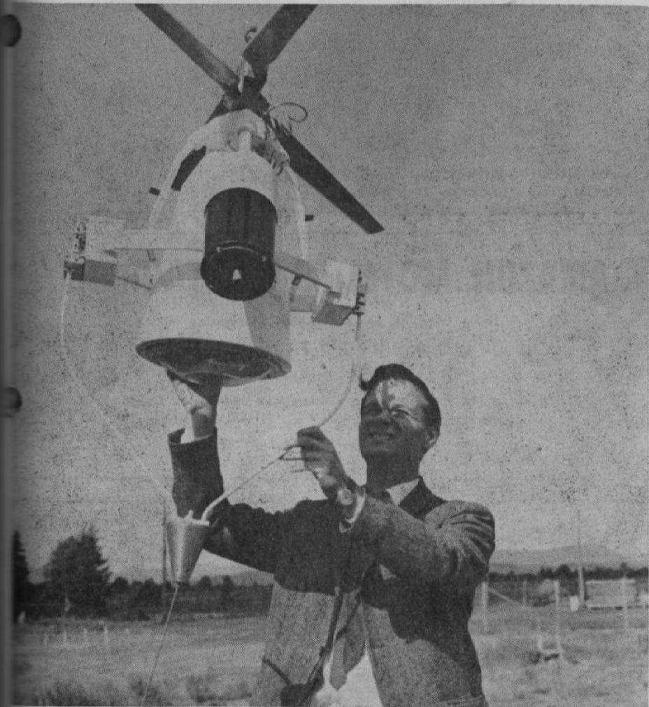
Project engineer Christopher Wilson, of the Canadian Armament Research and Development Establishment, Valcartier, P.Q., demonstrates the lightness of the airborne component of the periscope, a CARDE-designed surveillance device. A winch on the control vehicle stores the tethering cable and permits raising and lowering of the airborne components.
