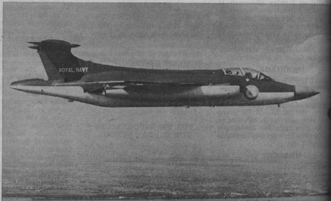
NEW BUCCANEER — A new version of the Buccaneer, the S2 in the flying programme at Farnborough. Powered by 2 Rolls-Royce Spey jets, the S2 is in full production for the British Royal Air Force. It has been designed as a high speed, low level strike aircraft capable of operating day or night, with conventional or nuclear weapons.
