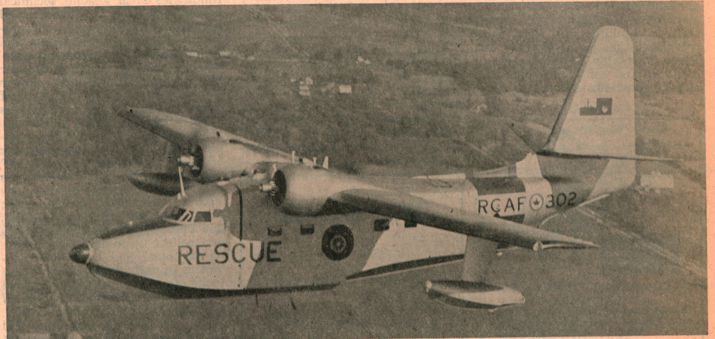
The "ALBATROSS," now in service with RCAF Search and Rescue units, is a general utility amphibian which can be used for air/sea rescue, as a hospital aircraft, or for photo reconnaissance work. Statistics: Length 62 ft. 4 in.; Wingspan, 96 ft. 6 in.; Weight, 32,000 lbs.; Speed 225 m.p.h.; Power, Two 1,425 h.p. Curtiss-Wright engines.
