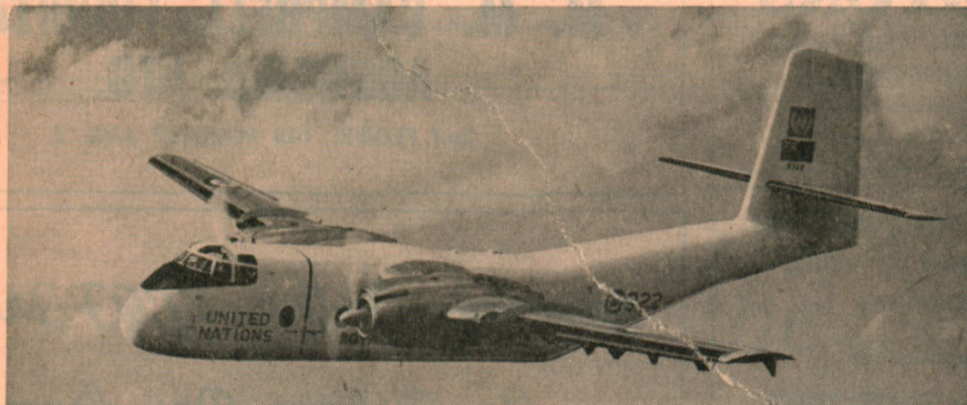
The "CARIBOU," designed for short runways, can take off fully loaded within 500 feet. It is now in RCAF service with the United Nations Emergency Force in the Middle East. Statistics: Length, 68 ft., 10 in.; Wingspan, 96 ft.; Weight 24,000 lbs.; Speed, 183 m.p.h.; Power, Two 1,450 h.p. Pratt and Whitney engines.
