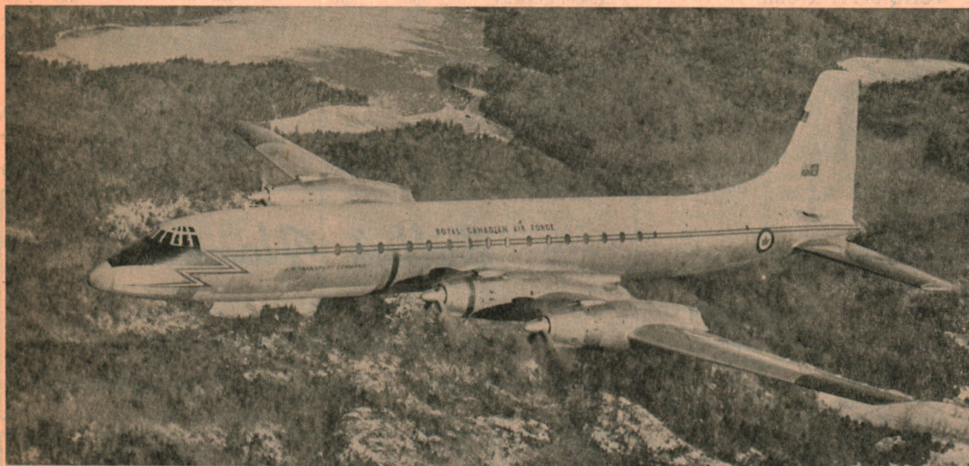
The CC106 is the largest aircraft built in Canada. Now going into service with the RCAF's Air Transport Command, the CC106 can carry a 30,000 lb. payload nearly 4,000 miles at 370 m.p.h., or a 55,000 lb. payload nearly 2,000 miles at the same speed. Statistics: Length, 136 ft. 8 in.; Wingspan, 142 ft. 3 1/2 in.; Weight, 155,000 lbs.; Power, Four 5730 h.p. Rolls Royce turboprops.
