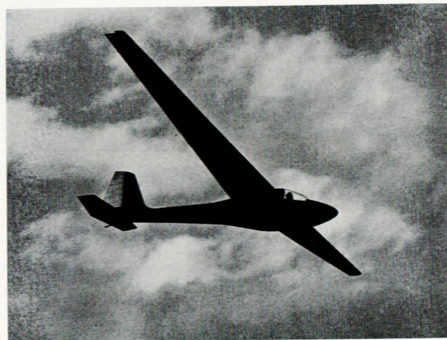
The Olympic 419 sailplane designed by the British firm of Elliotts of Newbury Ltd., Berkshire, England. A feature of this high performance sailplane is its 19-metres wing span.
