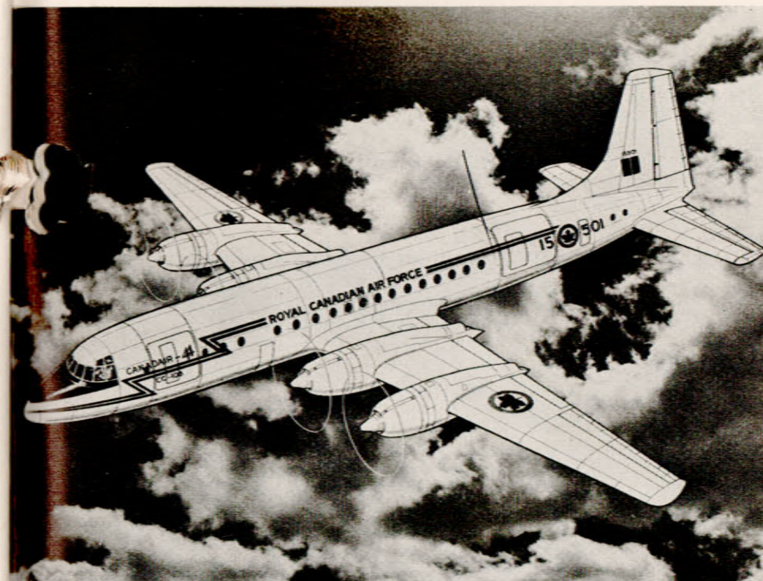
Artist's conception of the CL-44 turbo-prop transport now in production for the RCAF in one of Canadair's Montreal plants.
