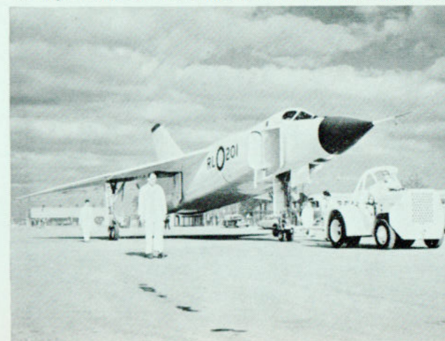
The Avro Arrow is as big as a World War II bomber yet took off on its first flight in only 3,000 feet of the 11,000 foot runway at Malton. ▼
