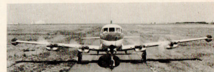
Cessna Aircraft Company's pressurized executive transport, the Model 620, is pictured with all four engines running shortly before the aeroplane started taxi tests. No date for the maiden flight has been set, according to Cessna officials.
