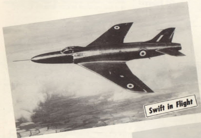
The "Swift", first swept wing jet fighter to go into production for the RAF, carries on the close association of Rolls Royce and Supermarine companies. The famous Spitfire was powered by a Rolls Royce piston engine and in like manner the "Swift" is driven by the Rolls Royce Avon jet engine. The Rolls Royce, Supermarine combination won for Britain the Schneider Trophy with the S6B.
