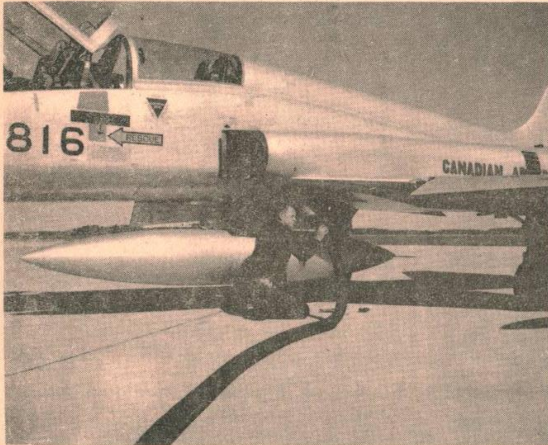
Single point, high pressure refuelling resulted in a turnaround at Gimli of 6:15.
