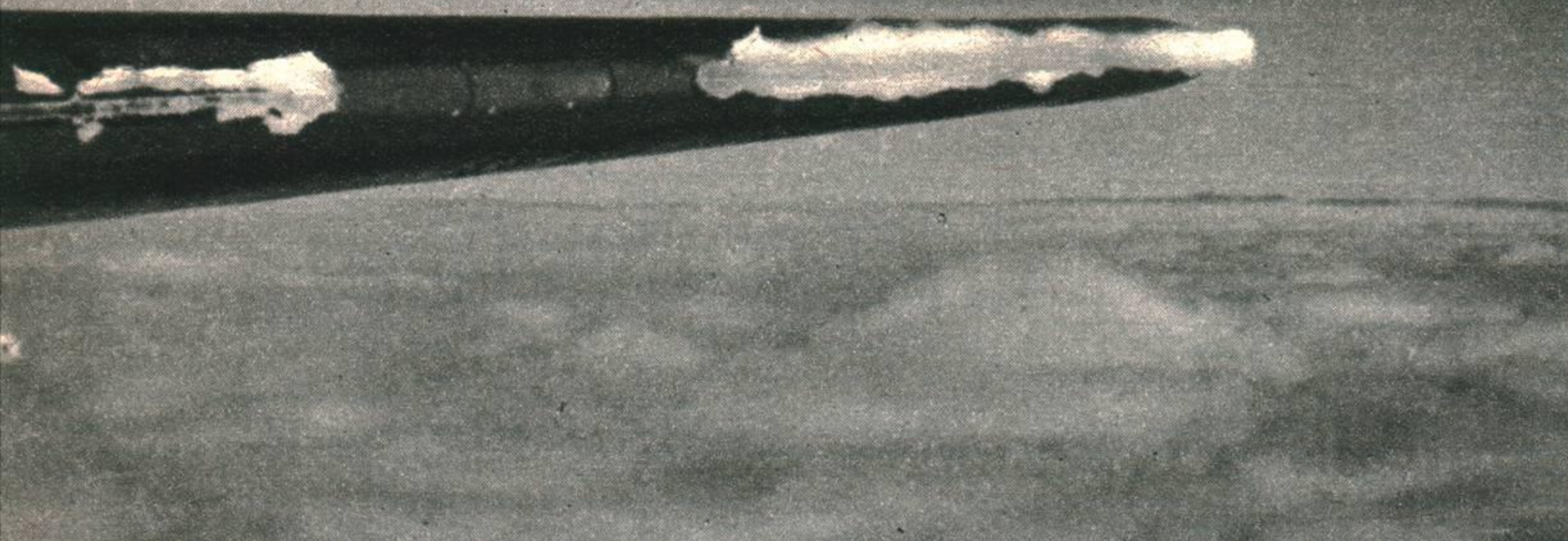
These photographs of the port and starboard tailplanes of the Viking in which the B.E.A. de-icing flight trials were conducted clearly demonstrate the effectiveness of the Porosint panel distributors as against the standard strip-type distributors (immediately inboard) and also indicate, by the ice accretion on the unprotected outer portions of the leading edges, the severity of the icing conditions encountered.
