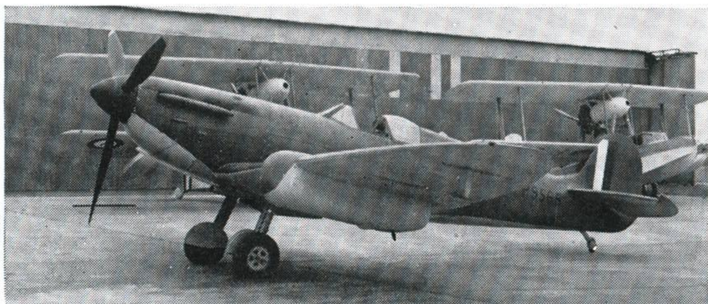
Spitfire IIA P9565 with a 40-gallon long-range fuel tank on the port wing (Type 343).
