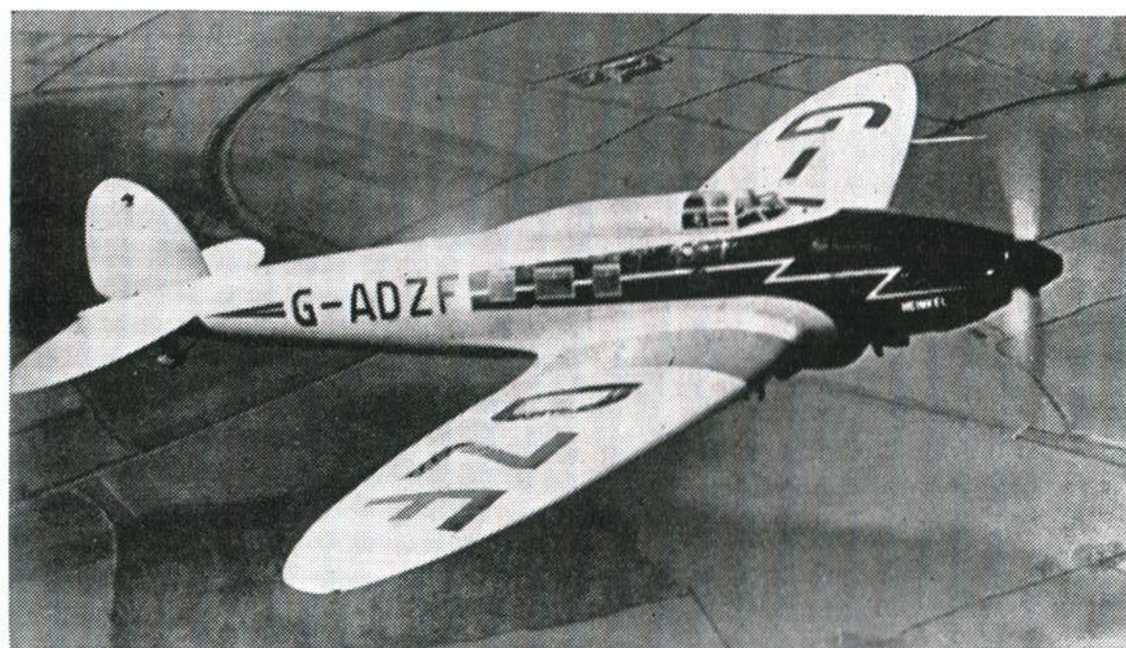
The sleek Heinkel He.70 (actually the example used by R-R as a Merlin test-bed) and (below) the prototype Type 300 Spitfire whose design the German aircraft greatly influenced.
