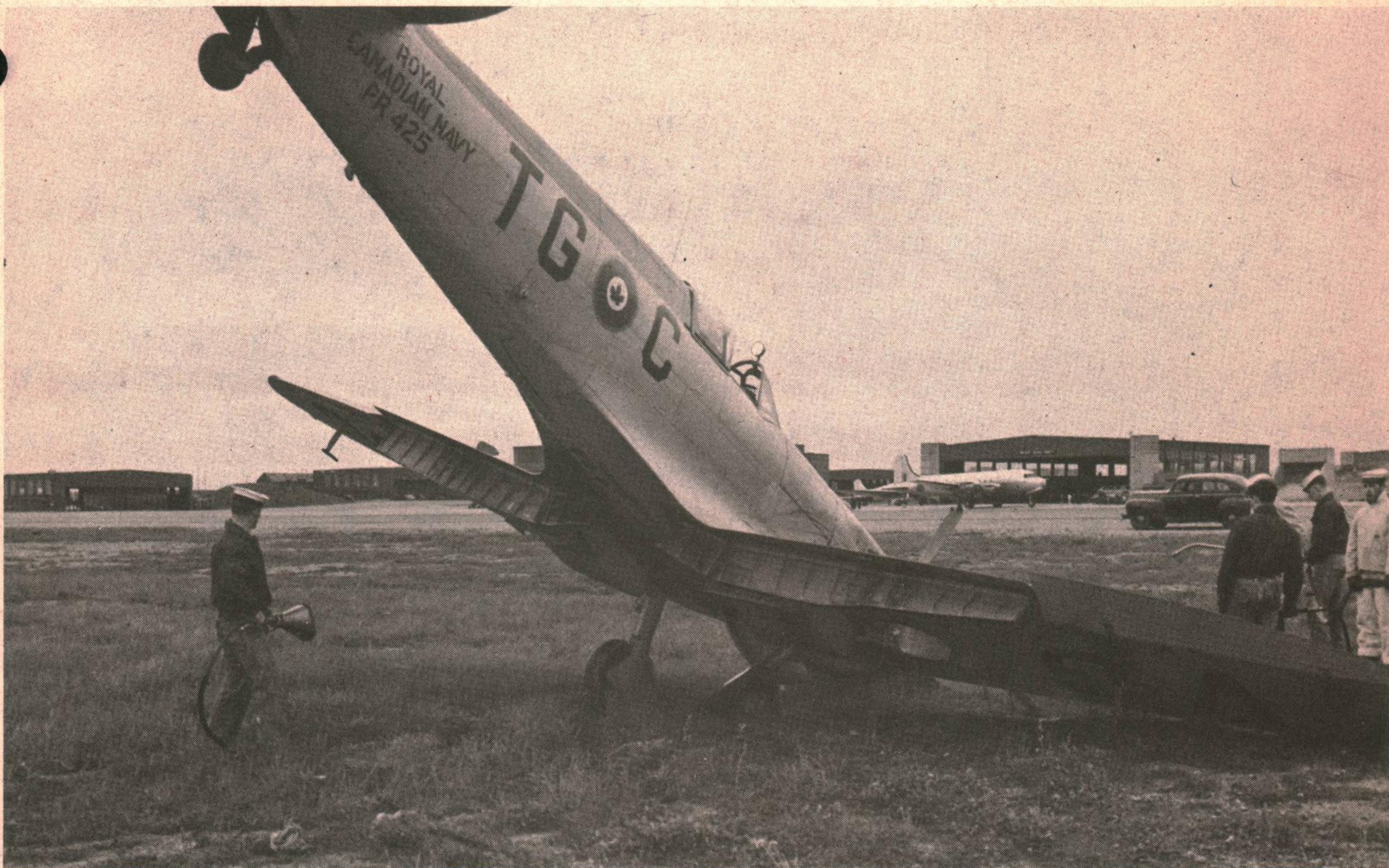
Pranged Seafire XV. PR425 piloted by Lt. Barge destroyed its right gear leg and went up on its nose at Dartmouth on 14 June 1948. Note the fully dumped flaps. (Public Archives of Canada/DNS-374)
