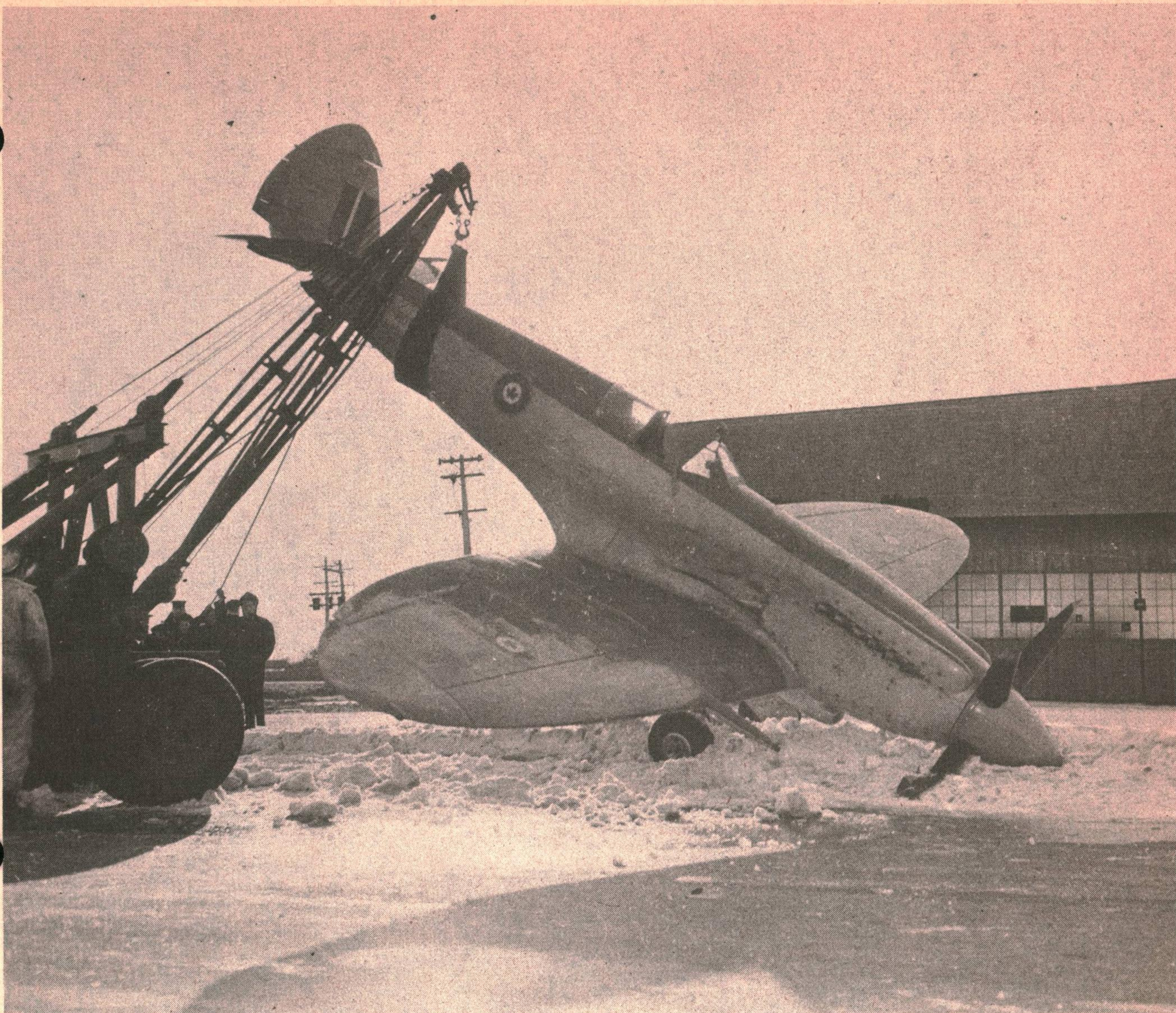
Seafire XV PR470 of Lt. M. T. Geary of No. 803 Squadron after nosing over in snow while taxiing at RCN Dartmouth on 19 February 1948. Compare the paint scheme in this photograph with the opening view of PR470. Note the use of very small roundels on the wing and fuselage. The Seafire XV was created by using a basic Spitfire VB fuselage with LIII folding wings and the enlarged fin and rudder of the Spitfire VIII with that version's retractable tail-wheel, wing-root fuel tanks from the Spitfire IX, the Spitfire XII's engine installation and auxiliaries but with a completely navalized Griffon engine. (Public Archives of Canada/DNS-224)
