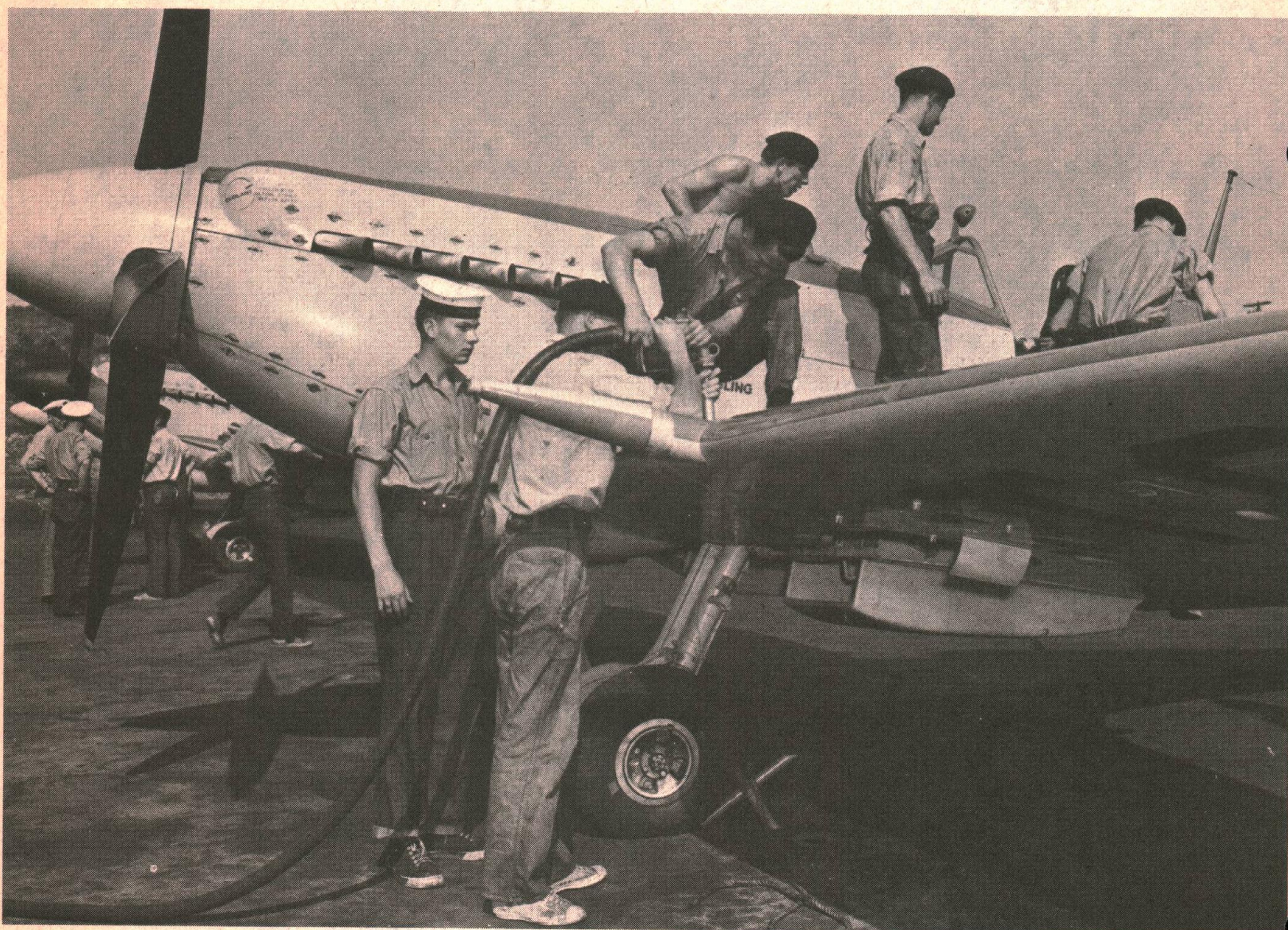
Good overall view of a Mk.XV being serviced and fueled. Note the very small size of the Seafire. Note how the fairing on the cannon barrel has been refitted upside down. The Canadian Seafires
