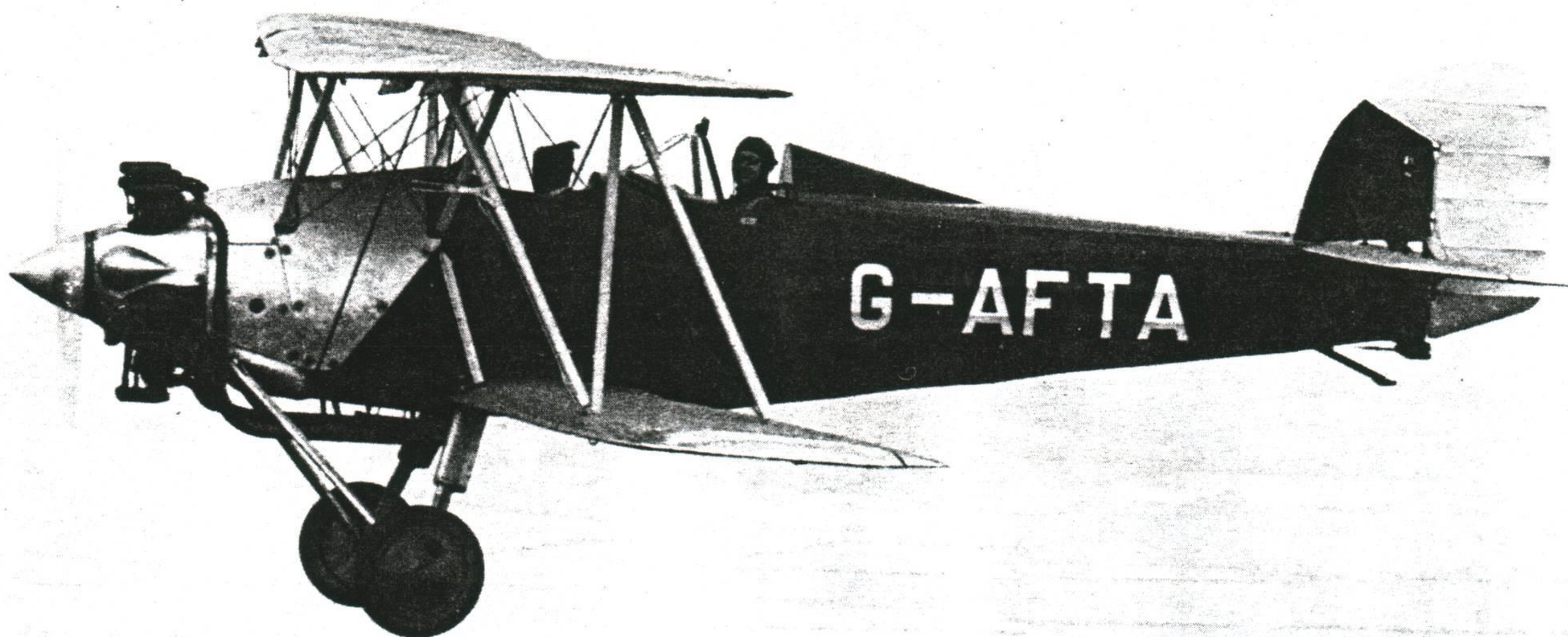
G-AFTA was the final Tomtit to be built, and was flown by Hawker test pilot Neville Duke for a while. Note the exposed cylinders and crankcase fairing and the attractive vintage look of the aircraft
